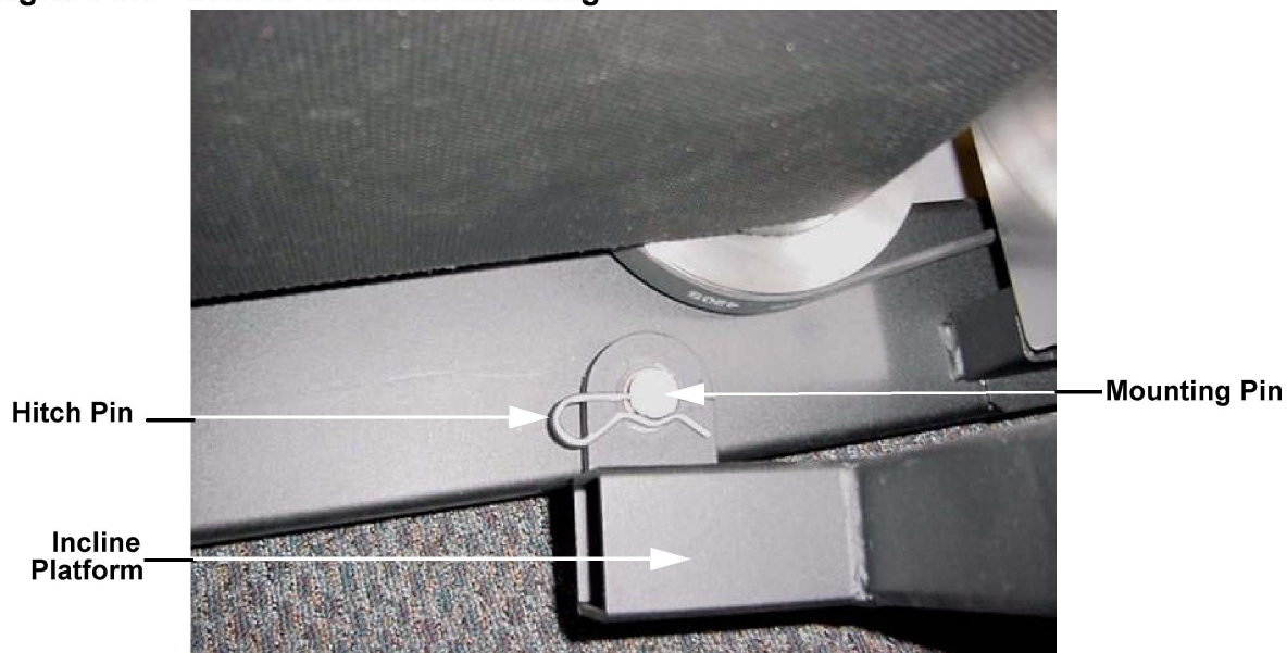
Diagram 6.1 - Incline Platform Mounting
